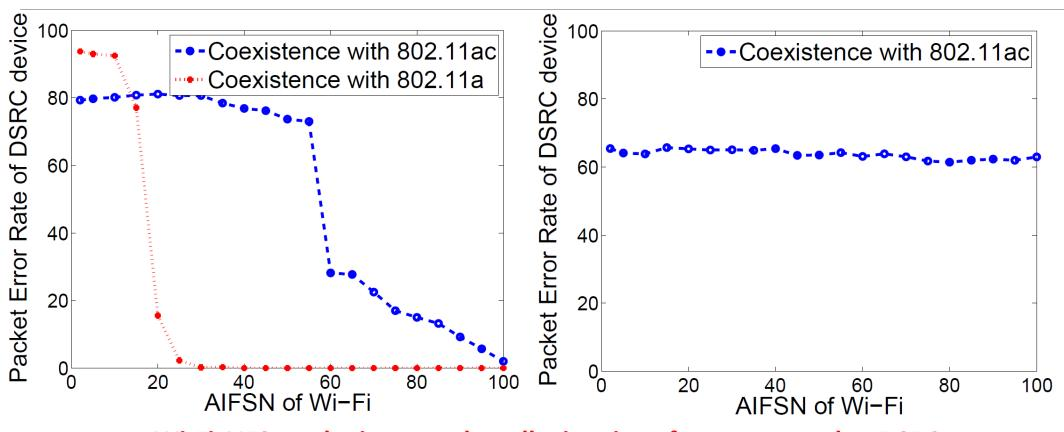
Wi-Fi AIFS can be increased to alleviate interference caused to DSRC DSRC nodes operating in secondary Wi-Fi channels suffer significant degradation
