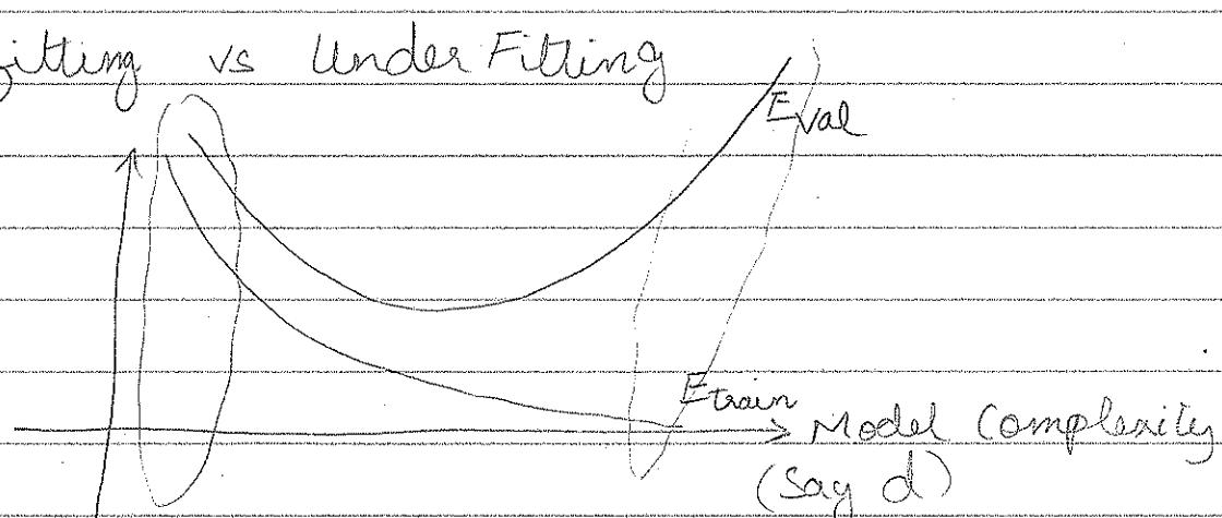
$\text{Eval} \approx \text{Etrain} = \text{high} \Rightarrow \text{Underfitting}$
