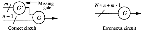
Figure 3 The missing-gate design error (MGE).
