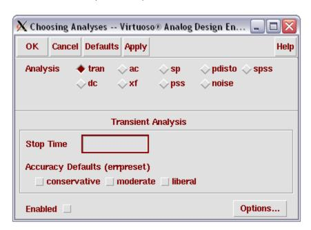
i. If you chose the dc or ac analysis, which are equivalent to the DC or AC Sweep in OrCAD PSpice and you chose to sweep a Component Parameter, you will then have to Select Component. Click on this button and then click on the component symbol in the Virtuoso Schematics Editing window.
