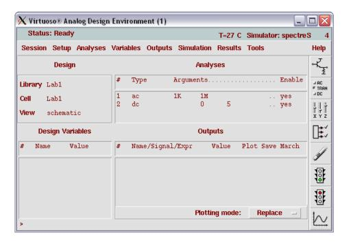
d. To identify which outputs should be plotted at the end of the simulation, click on **Outputs** → **To Be Plotted** → **Select On**
