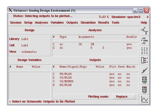
e. To run the simulation, select **Simulation** → **Run** on the upper toolbar of the **Analog Design Environment** window or click on the icon on the right. A plot of the outputs should be displayed at the end of the simulation.
