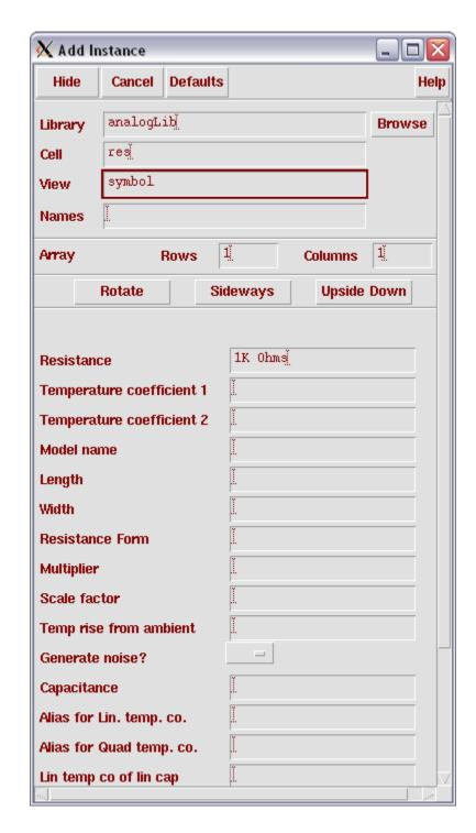
f. Now move your mouse on to schematic in the **Virtuoso Schematic Editing** window. The symbol of the part that you selected should appear.
